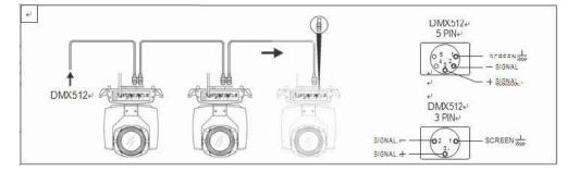
Figure 1 DMX Cable connection
